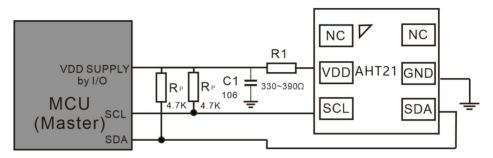
Figure 15. Typical application circuit.
