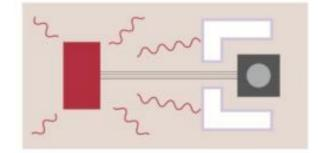
Figure 14. The sensor is isolated from the internal heat source to minimize the effect of internal heat on sensor.
