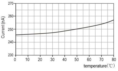
**Figure 6**. Typical supply current vs. temperature curve (sleep mode) when VDD=3.3V. Please note that there is a deviation of approximately  $\pm 25\%$  between these data and the displayed value.
