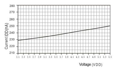
**Figure 7** The relationship between typical supply current and supply voltage at 25 °C Curve (sleep mode), please note that the deviation of these data from the displayed value may reach ±50% of the displayed value. At 60 °C, the coefficient is about 15 (Compared with table 2)
