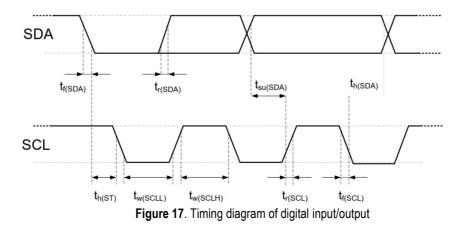
The abbreviations are explained in Table 8. The thicker SDA line is controlled by the sensor, and the ordinary SDA line is controlled by the single-chip microcomputer. Please note that the SDA valid read time is triggered by the falling edge of the previous conversion.
